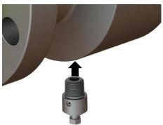
✓ Installation of the safety plug is now complete.
