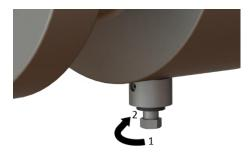
✓ The safety drain plug is open and the fluid residues can escape.
