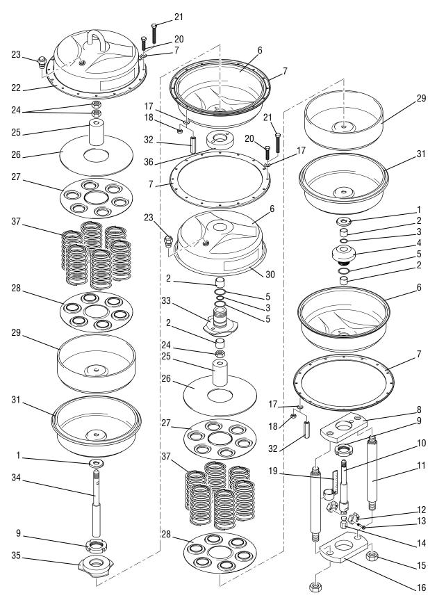
Fig. 1: Series 5 On-Off Actuator, Air-to-Open
