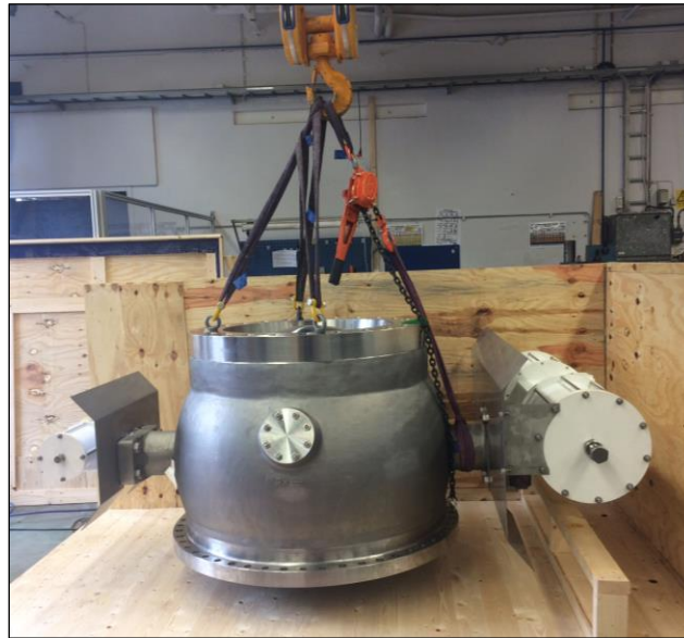
Figure 2: Lifting of a NAF ProCap with mounted actuators.
