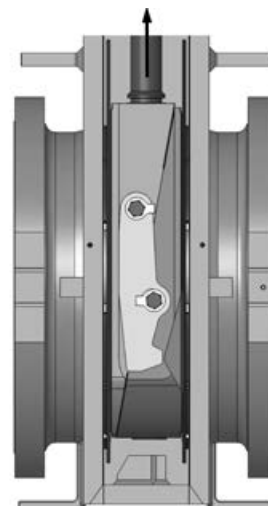
Figure 7b: Gate and segment contracted by connected arm
