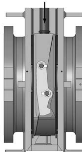
Figure 7a: Gate and segment expanded against seats
