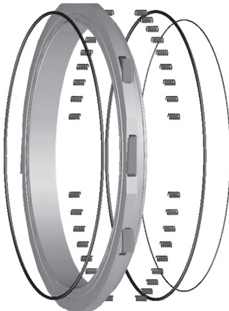
Figure 18 - Seat gaskets and springs stripping.
