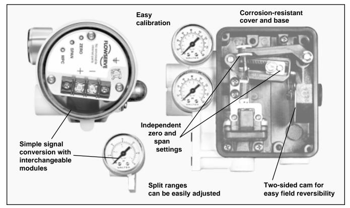
Figure 1: Features of Beta Positioner with Pneumatic or Electro-pneumatic modules
