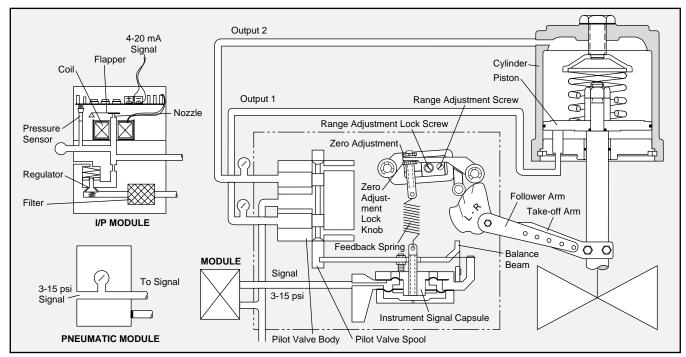
Figure 4: Positioner Schematic for Air-to-Open (Retract)
