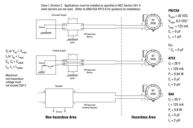
Figure 2 – NT 3000 Transducer Schematic
