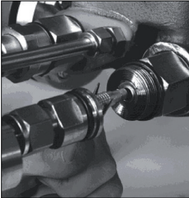
Figure 10: Disconnecting Lemo™ Connector
