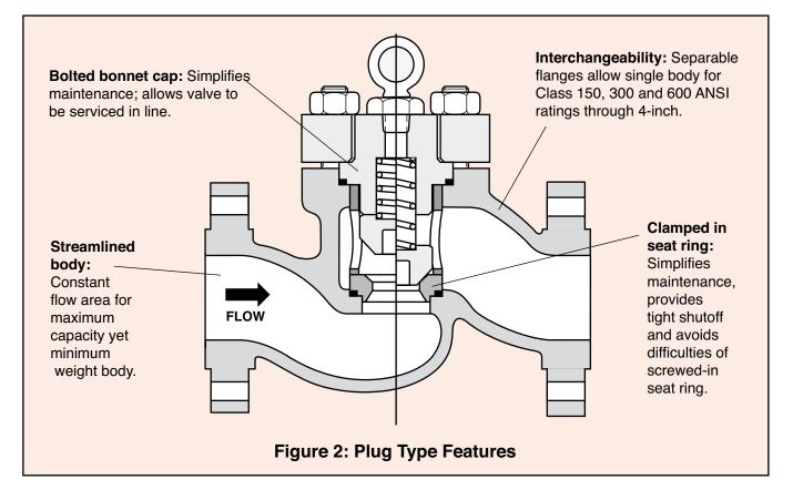
Similar in some respects to the non-slam design, the Tek-Check, plug-type check valve is designed for applications requiring quick shutoff. Due to its simple design, the plug-type check valve costs less and has fewer parts than the non-slam check valves.
