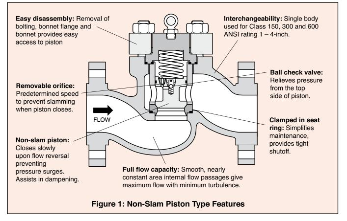
The Valtek Tek-Check<sup>™</sup>, non-slamming piston check valve, provides rugged performance and reliable service in corrosive and non-corrosive, gas and liquid applications. The smooth, nearly-constant area internal passages allow for high capacity flow with minimum turbulence. When the flow ceases or is reversed, the piston closes slowly, preventing pressure surges. The non-slam design is also effective in dampening pulsating flow.
