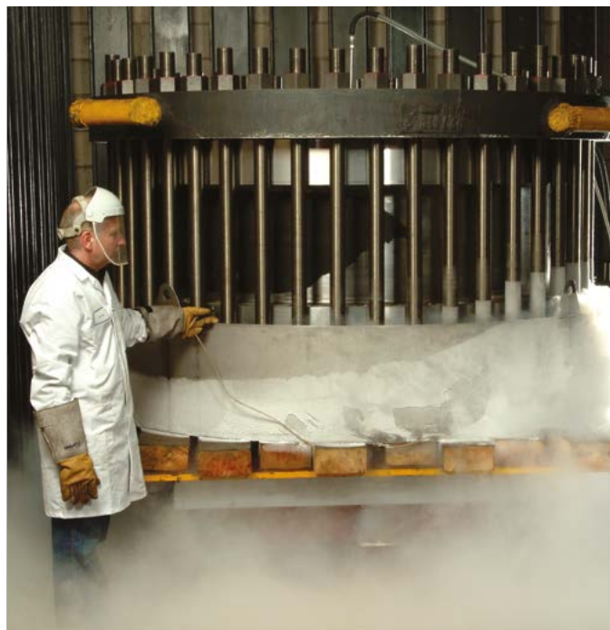
Cryogenic test facility for helium leak testing
