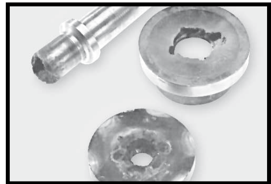
Figure 5: Cavitation Damaged Parts
