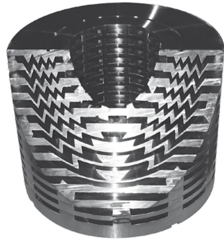
Figure 4.2: Cross-Sectioned TigerTooth Seat Retainer
