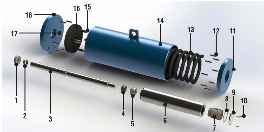
Figure 22: Spring Can Exploded View
