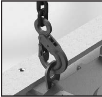
Figure 1a: Use of Lifting Lug
