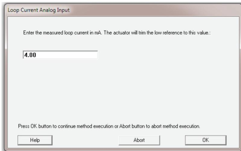
Enter the measured value of the loop current in mA that was applied in the previous step.
