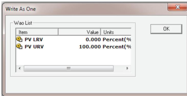
To change the upper range value, click on a PV URV item; a new window will open, allowing the user to enter the value.
