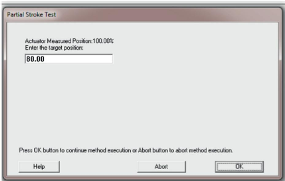
Enter the target position you wish the actuator to move to (it will return to the start position after it reaches the target position). The current start position is displayed as “Actuator Measured Position”
