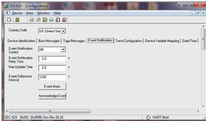
The Event Mask allows the user to select those bits from Field Device Status and Command 48 data which they want to trigger and event. When the user clicks the “Event Mask” button, the following menu will appear, allowing them to select the event triggers:
