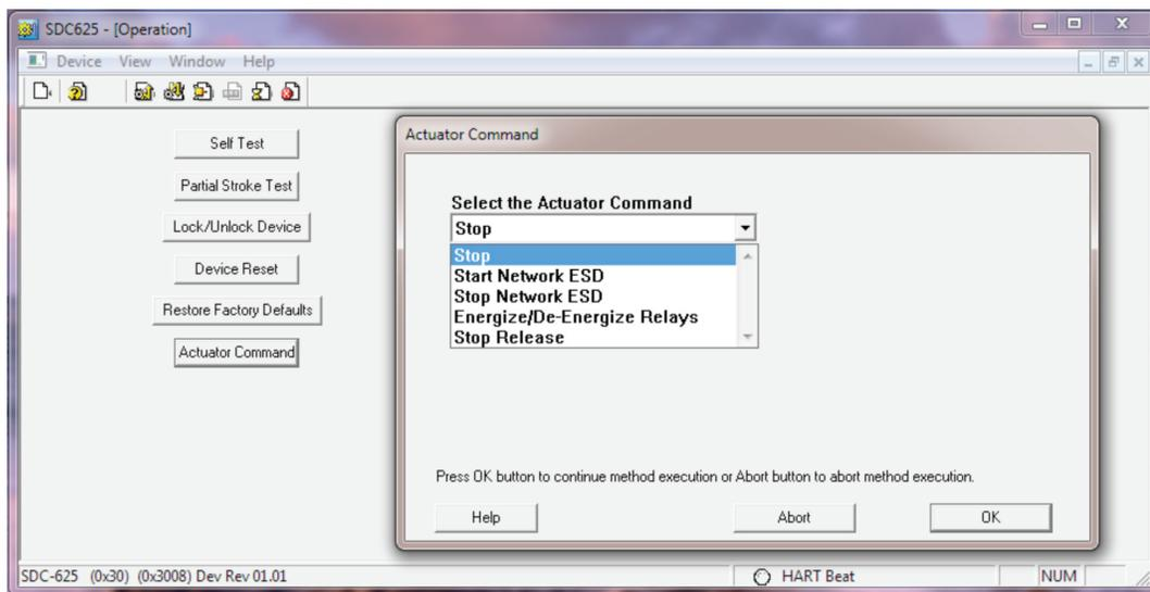
The Stop and Stop Release commands require the unit be in Remote; if not, in remote response code 16 “Access Restricted” will be returned. The Stop command is used like a network stop and will halt the unit from reacting to the PV value. The Stop Release command will remove the network stop and resume normal operation.
