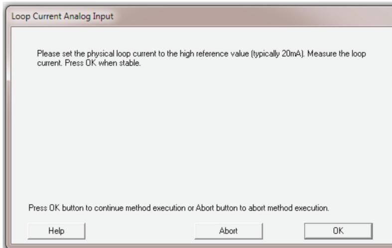
Set the Analog Input Loop Current to the high reference value (typically 20 mA, but can be set between 12-28 mA) and then click OK.
