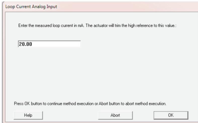
Enter the measured value of the loop current in mA that was applied in the previous step.
