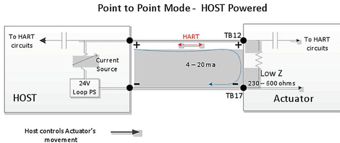
Figure 2.4 – Point-to-Point Topology (Loop Powered)
