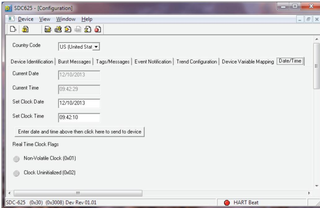
The MXa/QX HART Device does not support a Non-Volatile Clock, therefore, if power is lost or the unit resets, the date and time are lost and must be reset.
