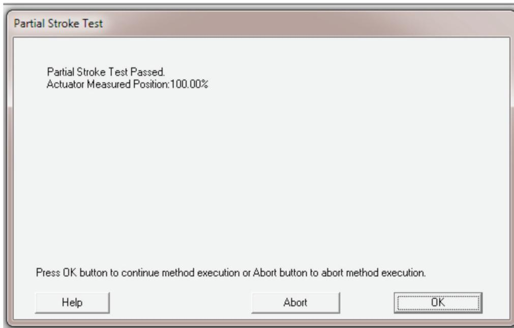
If the test failed, “Partial Stroke Test Failed” would be displayed and further information on the failure can be found by reviewing the DD menu Diagnostics->Information->Device Status.
