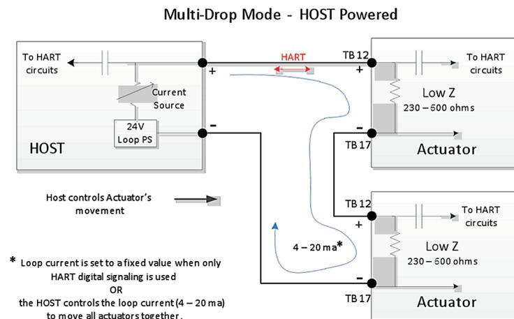
Figure 2.6 – Multi-drop Topology (Loop Powered)
