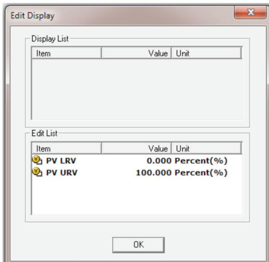
The current Lower (LRV) and Upper (URV) ranges are shown. To change the range value, click on the item to be changed; a new window will open, allowing the user to set both limits at the same time.
