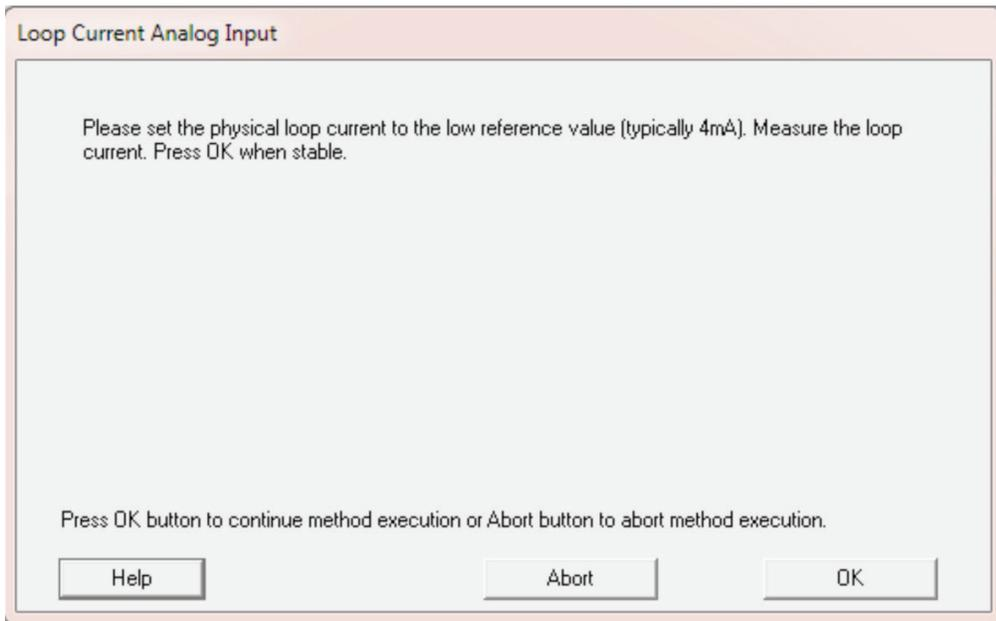
Set the Analog Input Loop Current to the low reference value (typically 4 mA, but can be set between 2-7 mA) and then click OK.
